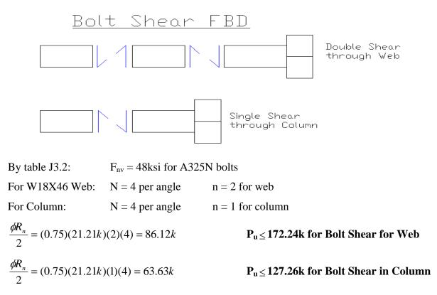
To calculate shear rupture, we followed equation (J4-4). The angles were assumed to be A36 steel with a yield strength of 36 ksi, and an ultimate strength of 58 ksi. The angles used in the connections are L4 x 4 x 3/8. The following calculations were used to determine the bearing capacity of the angles.
