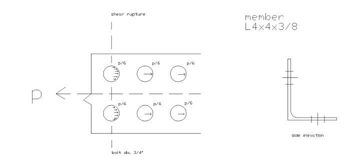
$\frac{\Phi R_n}{2} = 0.75*38.625 \ kips = 28.971 \ kips$  per angle
