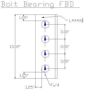
By table J3.4  $L_{e \min} = 1 \frac{1}{4} in L_{e \max} = (1.5(d_{bolt}), L_e)$   $Le = 1 \frac{1}{4} in$ Edge Bolts:  $L_c = 1 \frac{1}{4} in$
