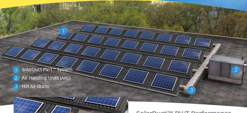
The SolarDuct™ product can also be used for PV/ thermal cogeneration systems. With a SolarDuct PV/T system, the all-metal SolarWall® panels draw the heat away from the PV modules. This heat energy is then ducted to the nearest rooftop air handling unit and then into the building's conventional HVAC system where it offsets the heating load.
