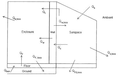
Fig. 1. Schematic of passive-solar residence.
