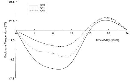
Fig. 3. Enclosure temperature response to optimal control for sunny day.
