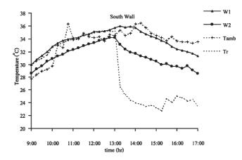
Fig. 6. Variation of temperatures of masonry wall of common house when the AC is turned on at 1 p.m. (average ambient condition:  $539 \text{ W/m}^2$ , 33.54 °C; 8/5/00).
