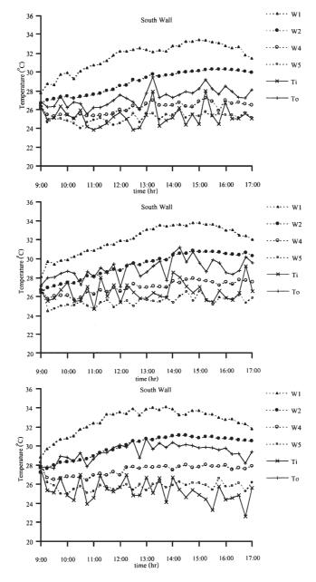
Fig. 16. Variation of temperatures at different positions of open south side MTW. Top:  $75 \times 5 \text{ cm}^2$  (average ambient condition: 512.48 W/m<sup>2</sup>, 32.71 °C; 20/6/00); middle:  $37.5 \times 5 \text{ cm}^2$  (average ambient condition: 469.38 W/m<sup>2</sup>, 32.39 °C; 23/7/00); bottom:  $5 \times 5 \text{ cm}^2$  (average ambient condition: 499.51 W/m<sup>2</sup>, 32.07 °C; 17/8/00).
