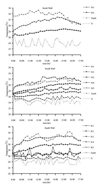
Fig. 4. Variation of temperatures at different positions of south wall. Top: common wall (average ambient condition: 492 W/m<sup>2</sup>, 33.38 °C; 6/5/00); middle: MTW with closed opening (average ambient condition: 531 W/m<sup>2</sup>, 30.82 °C; 18/7/00); bottom: MTW when opening (75  $\times$  5 cm<sup>2</sup>) are opened (average ambient condition: 411.94 W/m<sup>2</sup>, 32.01 °C; 20/7/00).
