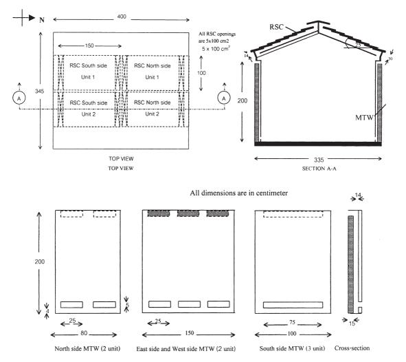
Fig. 1. Dimensions of roof solar collector and modified trombe wall (not to scale).
