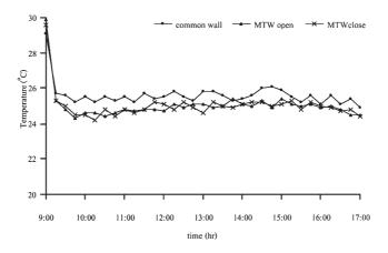
Fig. 10. Comparison of globe temperatures between common house (average 25.49 °C ,6/5/00), closed all RSC and MTW openings (average 24.89 °C, 14/6/00) and opened all SC (average 24.89 °C, 15/6/00).
