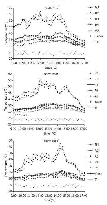
Fig. 3. Variation of temperatures at different positions of north roof. Top: common roof (average ambient condition: 492 W/m<sup>2</sup>, 33.38 °C; 6/5/00); middle: RSC with closed opening (average ambient condition: 462 W/m<sup>2</sup>, 33.97 °C; 14/6/00); bottom: RSC when opening ( $100 \times 5 \text{ cm}^2$ ) are opened (average ambient condition: 469.85 W/m<sup>2</sup>, 33.23 °C; 15/6/00).
