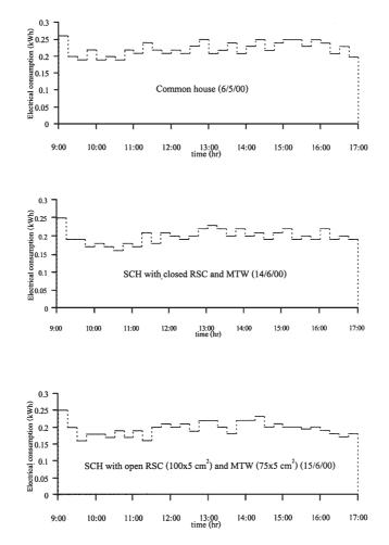
Fig. 13. Electrical consumption in 15 min intervals of AC for different test conditions.
