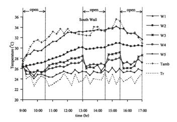
Fig. 5. Variation of temperatures of MTW when openings (surface area:  $75 \times 5$  cm<sup>2</sup>) are opened in intermittent mode: 9–10.30 a.m., 1–2.30 p.m. and 3.30–4.30 p.m. (19/8/00).
