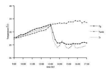
Fig. 12. Variation of globe temperature, ambient temperature and room temperature of SCH when AC is turned on at 1 p.m. with open all MTW ( $25 \times 5$  cm<sup>2</sup>, average ambient condition : 530 W/m<sup>2</sup>, 31.45 °C; 26/7/00).
