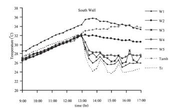
Fig. 7. Variation of temperatures of open MTW ( $25 \times 5 \text{ cm}^2$ ) when the AC is turned on at 1 p.m. (average ambient condition: 530 W/m<sup>2</sup>, 31.45 °C; 26/7/00).
