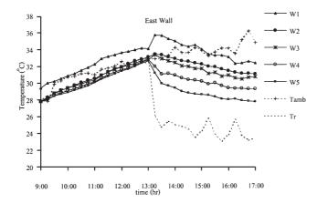
Fig. 8. Variations of temperatures of closed east-side MTW when the AC is turned on at 1 p.m. (average ambient condition: 465  $W/m^2$ , 32.54 °C; 28/7/00).
