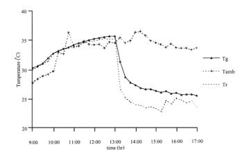
Fig. 11. Variation of globe temperature, ambient temperature and room temperature in common house when AC is turned on at 1 p.m. (average ambient condition: 539.40 W/m<sup>2</sup>, 33.54 °C; 8/5/00).
