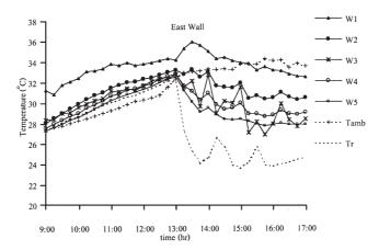
Fig. 9. Variation of temperature of open east-side MTW when the AC is turned on at 1 p.m. (average ambient condition:  $530 \text{ W/m}^2$ ,  $31.45 \text{ }^{\circ}\text{C}$ ; 26/7/00)
