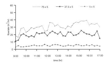
Fig. 15. Variation of air flow rate for different inlet openings of south MTW ( $75 \times 5 \text{ cm}^2$ , 20/7/00), ( $37.5 \times 5 \text{ cm}$ , 23/7/00) and ( $5 \times 5 \text{ cm}^2$ , 17/8/00).
