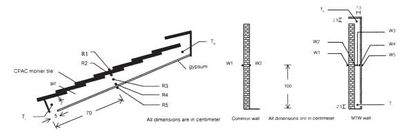
Fig. 2. Position of thermocouples setting in roof and walls (not to scale).
