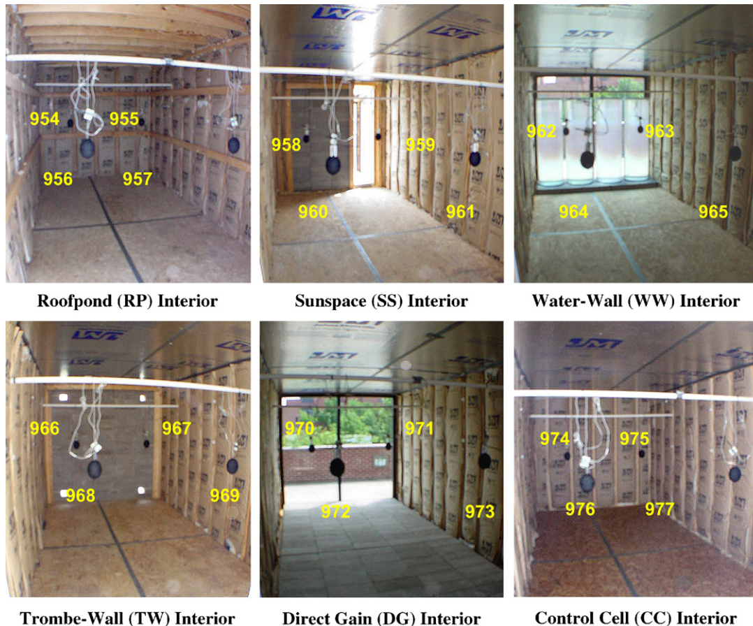
Fig. 3. Four-point grid used to monitor the indoor environmental conditions of the test-cells.
