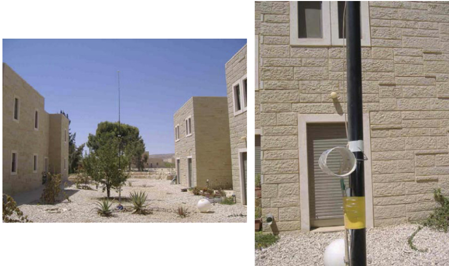
Fig. 12. Monitoring mast with shielded ultra-fine copper–constantan thermocouple placed in the middle of the street canyon.
