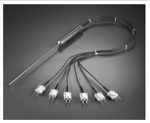
XACTPAK<sup>®</sup> mineral insulated, metalsheathed cable. Multipoint temperature sensors are available in either standard or special ASTM thermocouple calibration tolerances. For applications requiring extreme accuracy, special constructions can be made with platinum RTDs.
