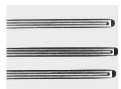
X-rays of the sensor verify the nonexistence of cracks at weld points that could let in humidity or gas and potentially shorten the life of the thermocouple.
