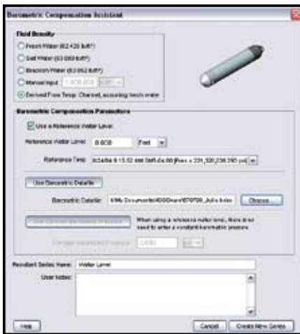
HOBOWare® software provides easy conversion to accurate water level readings, fully compensated for barometric pressure, temperature and water density.
