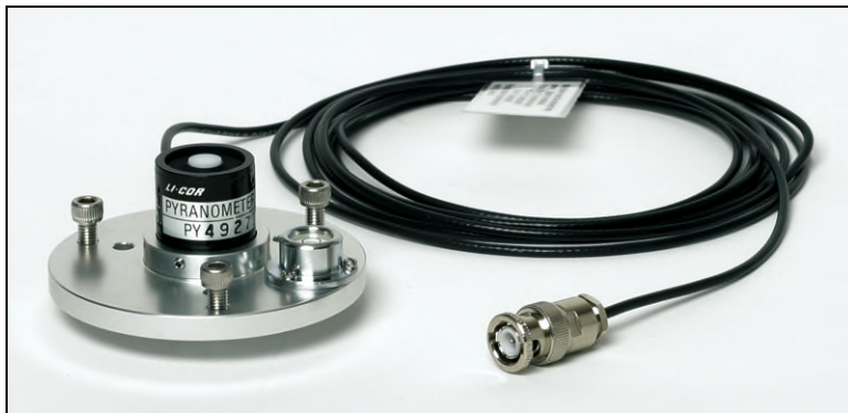
Figure 2-1. “SA” type sensors are terminated with only a BNC connector on the end of the coaxial cable.
