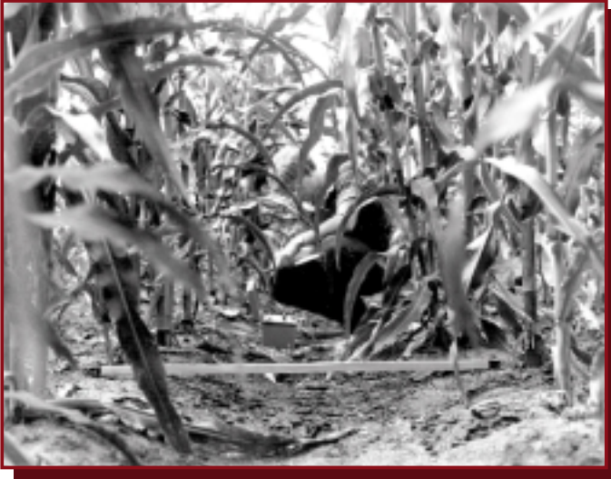
The LI-191SA Line Quantum Sensor spatially averages PPFD over its one meter length.
