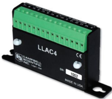
The LLAC4 mounts directly to the backplate of our environmental enclosures.
