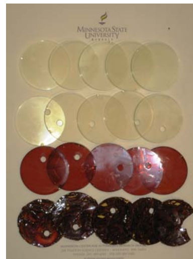
Figure 5. PUR samples (from top row to bottom row: non-immersed, Fuel C, E10, and E20)
