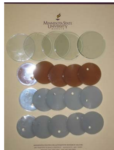
Figure 6. PVC samples (from top row to bottom row: non-immersed, Fuel C, E10, and E20)
