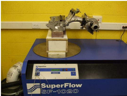
Intake runner flow and velocity testing.
