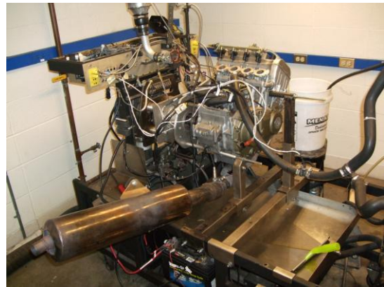
Engine run stand and dyno setup.
