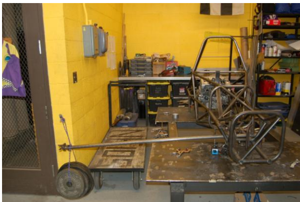
Physical torsion testing. 0.103" @ 600 lbf.
