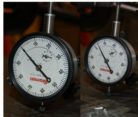
Before and after frame deflection.
