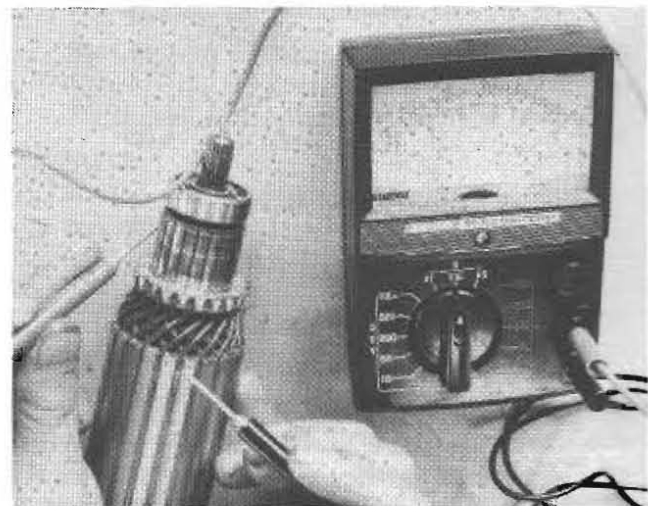
Fig. 6-10 Armature Ground Test
