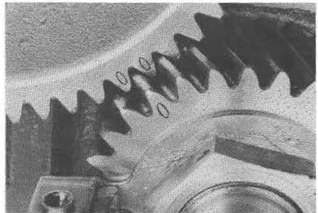
Fig. 4-12 Align Timing Marks
