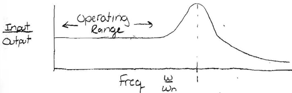
Assume  $\zeta = 1$  for damped response and  $\omega_n = 15000 \text{ Hz}$
