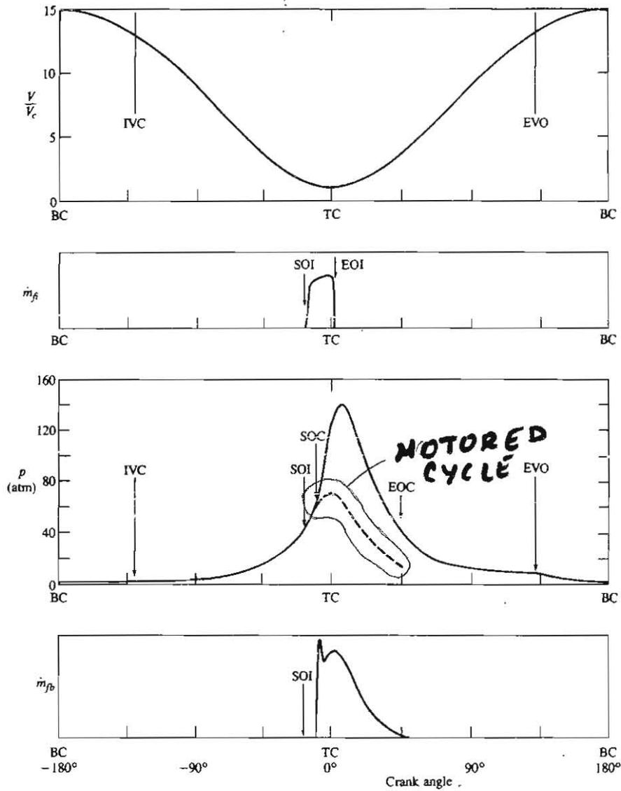
**FIGURE 1-15** Sequence of events during compression, combustion, and expansion processes of a naturally aspirated compression-ignition engine operating cycle. Cylinder volume/clearance volume  $V/V_c$ , rate of fuel injection  $\dot{m}_f$ , cylinder pressure  $p$  (solid line, firing cycle; dashed line, motored cycle), and rate of fuel burning (or fuel chemical energy release rate)  $\dot{m}_{fb}$  are plotted against crank angle.
