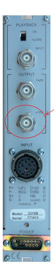
Connect to MTS analog input channel.
