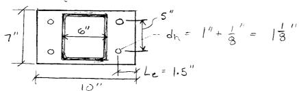
$$R_{n} \text{ per bolf} = r_{n} \left\{ \frac{1.2(1.5 - \frac{1}{2}(1.125))(\frac{3}{8})(58 \text{ ksi})}{2.4(1'')(\frac{3}{8})(58 \text{ ksi})} = 24.5 \text{ k} \right\}$$
