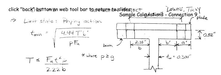
V 2T NOTE: the thickness of the flarge, to is 0.52", 2T while the plate thickness is 0.375". Also, the steel grade for the plate is lower (A36e vs A992), therefore.
