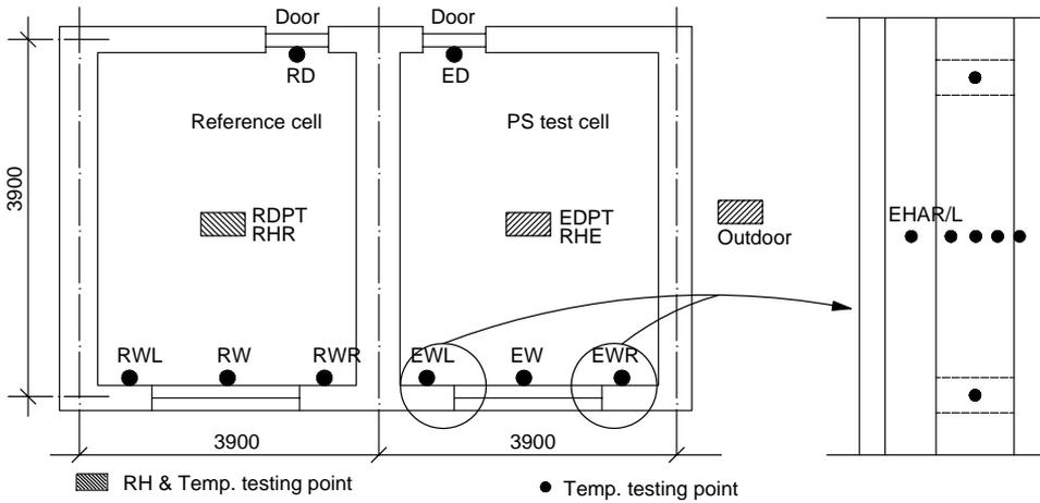
Fig. 3. Sketch map of RH and temperature testing points.
