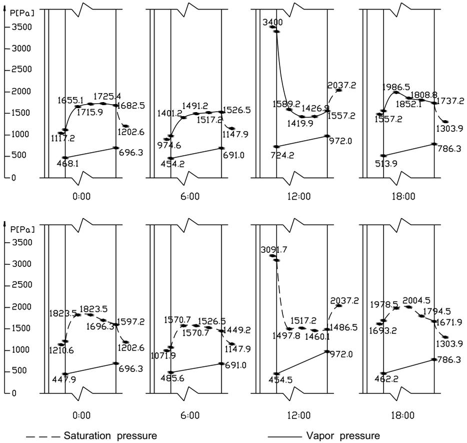
Fig. 8. Evaluation of condensation within Trombe walls of the PS cell at steady-state condition.
