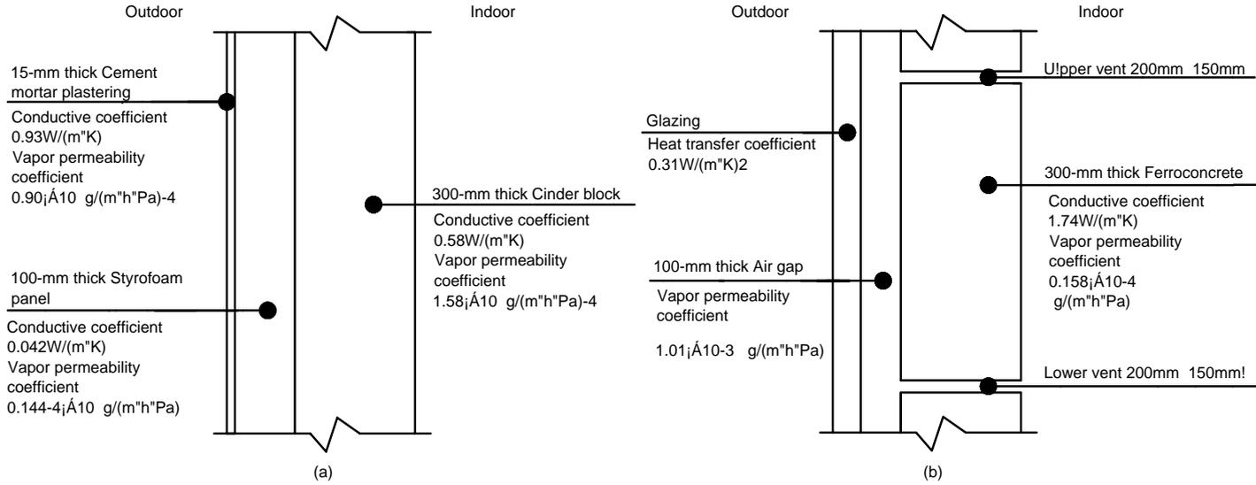
Fig. 2. Structure and physical parameters of the south facade walls. (a) Reference cell; (b) PS cell with Trombe wall.
