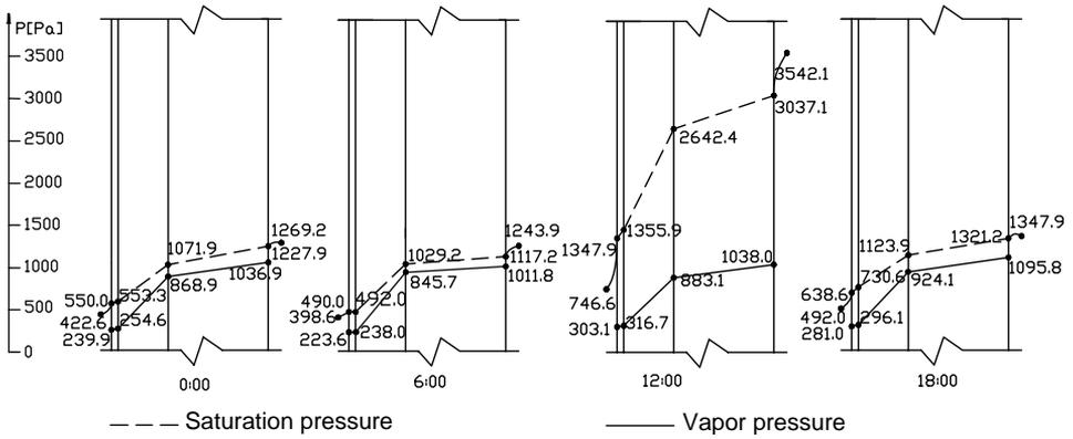
Fig. 7. Evaluation of condensation within the south facade wall of the reference cell at steady-state condition.
