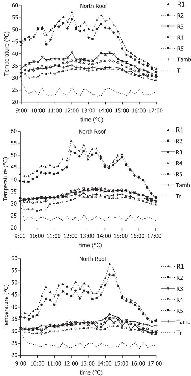
Fig. 3. Variation of temperatures at different positions of north roof. Top: common roof (average ambient condition:  $492 \text{ W/m}^2$ ,  $33.38 \text{ }^\circ\text{C}$ ; 6/5/00); middle: RSC with closed opening (average ambient condition:  $462 \text{ W/m}^2$ ,  $33.97 \text{ }^\circ\text{C}$ ; 14/6/00); bottom: RSC when opening ( $100 \times 5 \text{ cm}^2$ ) are opened (average ambient condition:  $469.85 \text{ W/m}^2$ ,  $33.23 \text{ }^\circ\text{C}$ ; 15/6/00).
