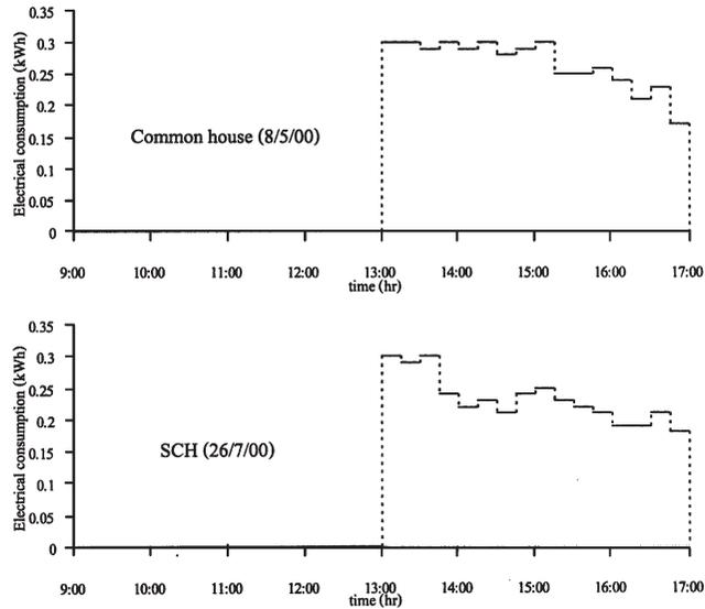
Fig. 14. Electrical consumption in 15 min intervals of of AC of common house and SCH turned on at 1 p.m. (26/7/00).
