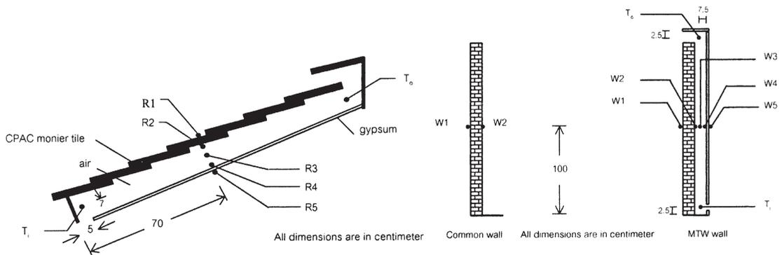
Fig. 2. Position of thermocouples setting in roof and walls (not to scale).
