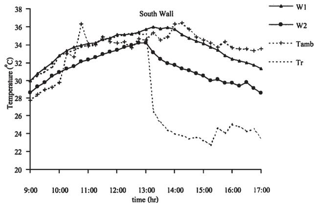
Fig. 6. Variation of temperatures of masonry wall of common house when the AC is turned on at 1 p.m. (average ambient condition:  $539 \text{ W/m}^2$ ,  $33.54 \text{ }^\circ\text{C}$ ; 8/5/00).
