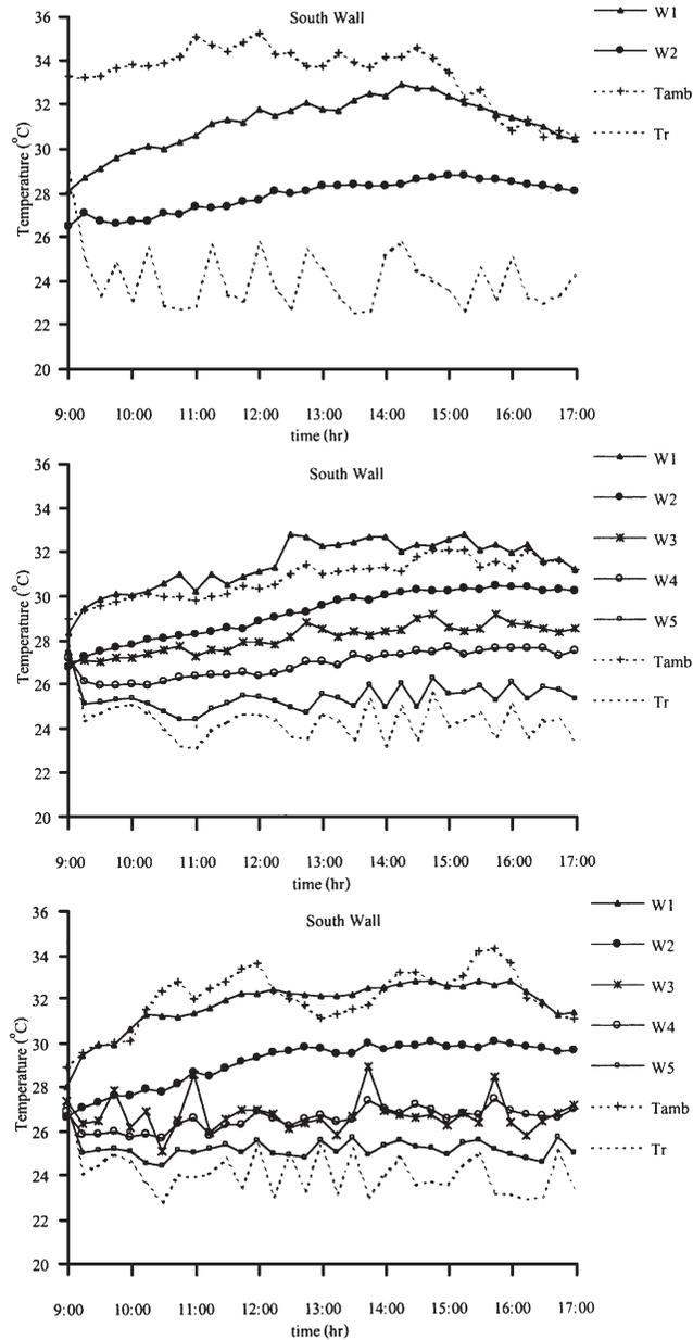
Fig. 4. Variation of temperatures at different positions of south wall. Top: common wall (average ambient condition: 492 W/m<sup>2</sup>, 33.38 °C; 6/5/00); middle: MTW with closed opening (average ambient condition: 531 W/m<sup>2</sup>, 30.82 °C; 18/7/00); bottom: MTW when opening (75 × 5 cm<sup>2</sup>) are opened (average ambient condition: 411.94 W/m<sup>2</sup>, 32.01 °C; 20/7/00).
