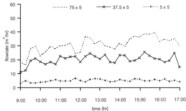
Fig. 15. Variation of air flow rate for different inlet openings of south MTW ( $75 \times 5 \text{ cm}^2$ , 20/7/00), ( $37.5 \times 5 \text{ cm}^2$ , 23/7/00) and ( $5 \times 5 \text{ cm}^2$ , 17/8/00).
