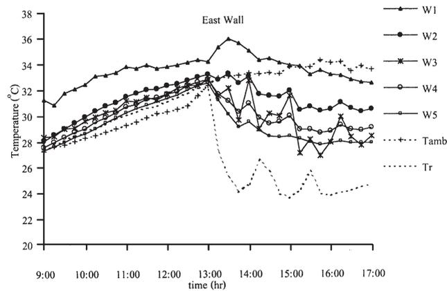
Fig. 9. Variation of temperature of open east-side MTW when the AC is turned on at 1 p.m. (average ambient condition:  $530 \text{ W/m}^2$ ,  $31.45 \text{ }^\circ\text{C}$ ; 26/7/00)
