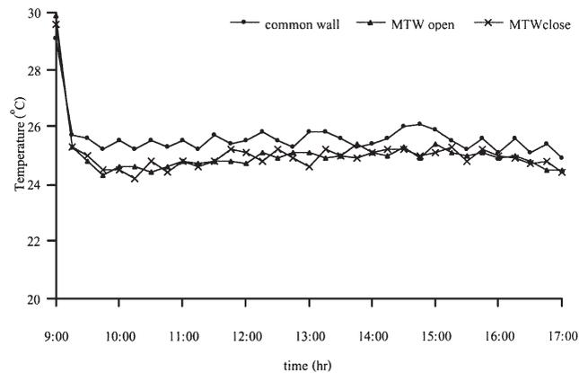
Fig. 10. Comparison of globe temperatures between common house (average  $25.49 \text{ }^\circ\text{C}$ , 6/5/00), closed all RSC and MTW openings (average  $24.89 \text{ }^\circ\text{C}$ , 14/6/00) and opened all SC (average  $24.89 \text{ }^\circ\text{C}$ , 15/6/00).
