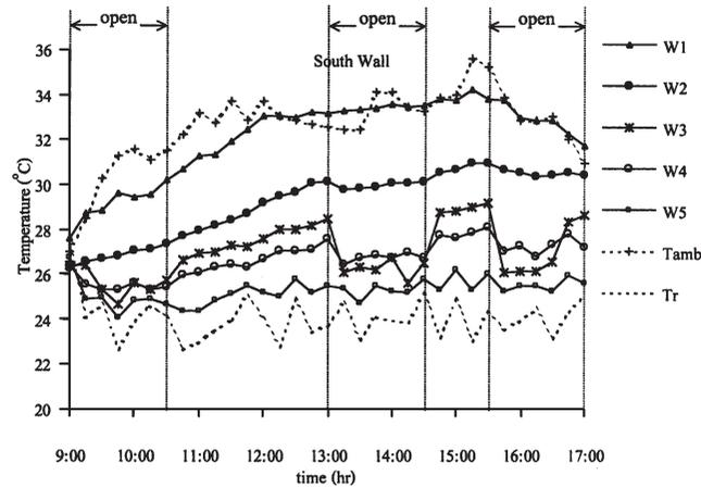
Fig. 5. Variation of temperatures of MTW when openings (surface area:  $75 \times 5 \text{ cm}^2$ ) are opened in intermittent mode: 9–10.30 a.m., 1–2.30 p.m. and 3.30–4.30 p.m. (19/8/00).
