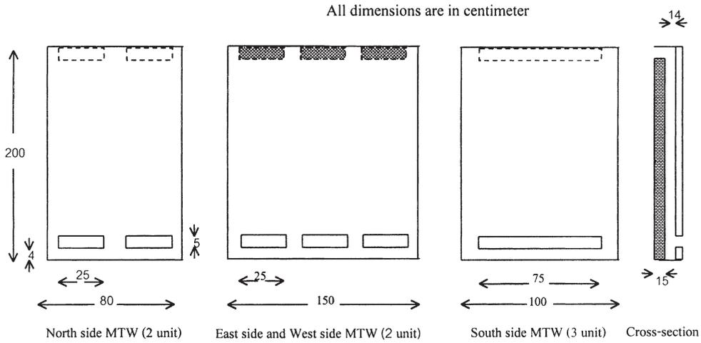
Fig. 1. Dimensions of roof solar collector and modified trombe wall (not to scale).
