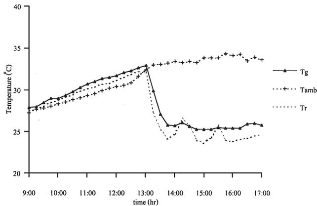
Fig. 12. Variation of globe temperature, ambient temperature and room temperature of SCH when AC is turned on at 1 p.m. with open all MTW (25 × 5 cm<sup>2</sup>, average ambient condition : 530 W/m<sup>2</sup>, 31.45 °C; 26/7/00).
