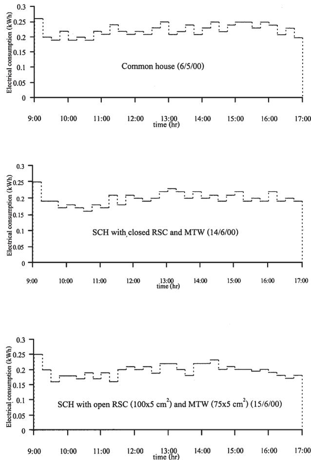
Fig. 13. Electrical consumption in 15 min intervals of AC for different test conditions.
