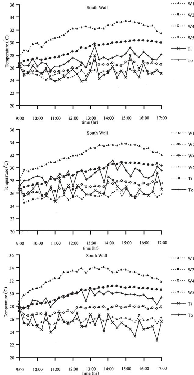
Fig. 16. Variation of temperatures at different positions of open south side MTW. Top:  $75 \times 5 \text{ cm}^2$  (average ambient condition:  $512.48 \text{ W/m}^2$ ,  $32.71 \text{ }^\circ\text{C}$ ; 20/6/00); middle:  $37.5 \times 5 \text{ cm}^2$  (average ambient condition:  $469.38 \text{ W/m}^2$ ,  $32.39 \text{ }^\circ\text{C}$ ; 23/7/00); bottom:  $5 \times 5 \text{ cm}^2$  (average ambient condition:  $499.51 \text{ W/m}^2$ ,  $32.07 \text{ }^\circ\text{C}$ ; 17/8/00).
