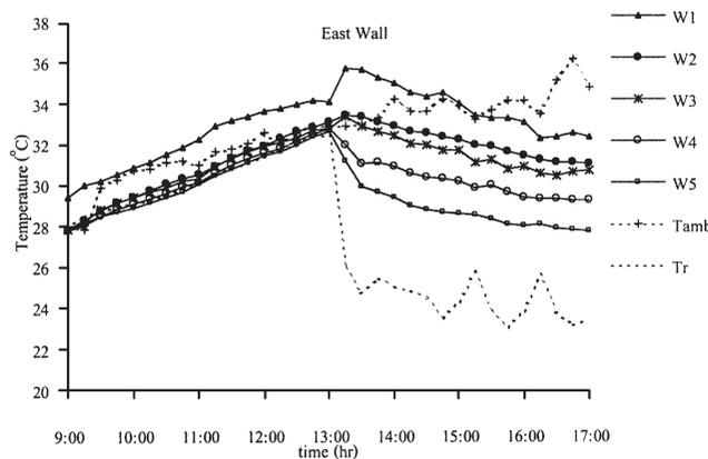
Fig. 8. Variations of temperatures of closed east-side MTW when the AC is turned on at 1 p.m. (average ambient condition:  $465 \text{ W/m}^2$ ,  $32.54 \text{ }^\circ\text{C}$ ; 28/7/00).
