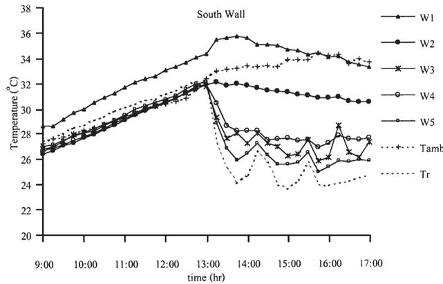
Fig. 7. Variation of temperatures of open MTW ( $25 \times 5 \text{ cm}^2$ ) when the AC is turned on at 1 p.m. (average ambient condition:  $530 \text{ W/m}^2$ ,  $31.45 \text{ }^\circ\text{C}$ ; 26/7/00).
