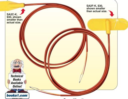
These sensors are available in 2 different mounting styles for flat or curved surfaces. The integral thermocouple sensor is bonded onto the inner surface of the self adhesive aluminum foil strip, which is provided for faster response times.
