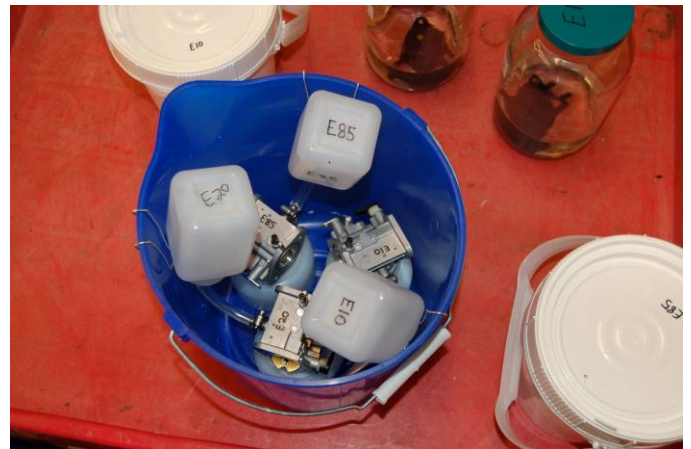
(Picture 8) Float Bowl specimens set up, ready for soaking.
