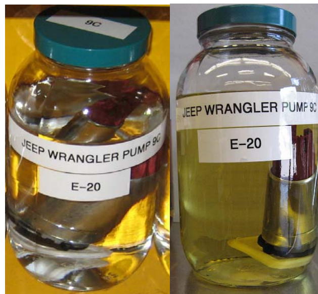
Figure 1. Jeep Wrangler Fuel Pumps (left E20 pre-immersion; right E20 post immersion)
