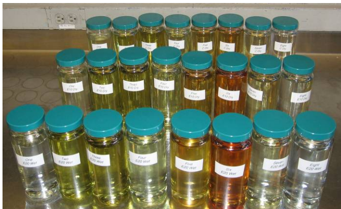
Figure 6. Discoloration comparison of the fuel after day 1 (front row E20; middle row E10; back row Fuel C)
