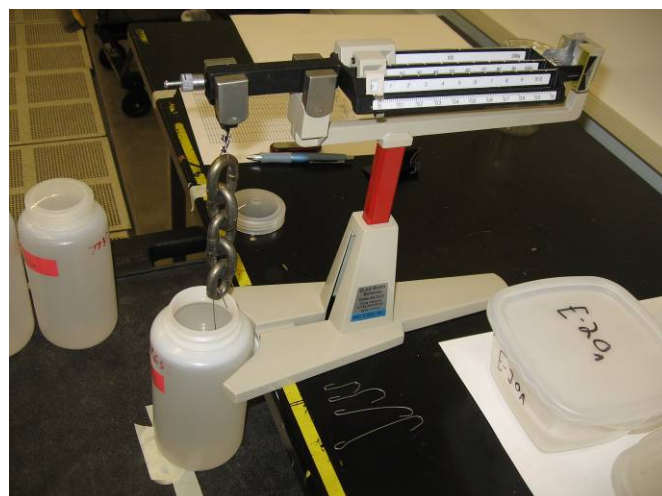
Figure 3. Quad beam balance used for volume measurements
