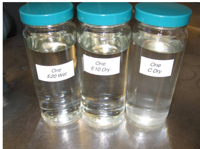
Figure 9. Cloudiness caused by ACM in Fuel C
