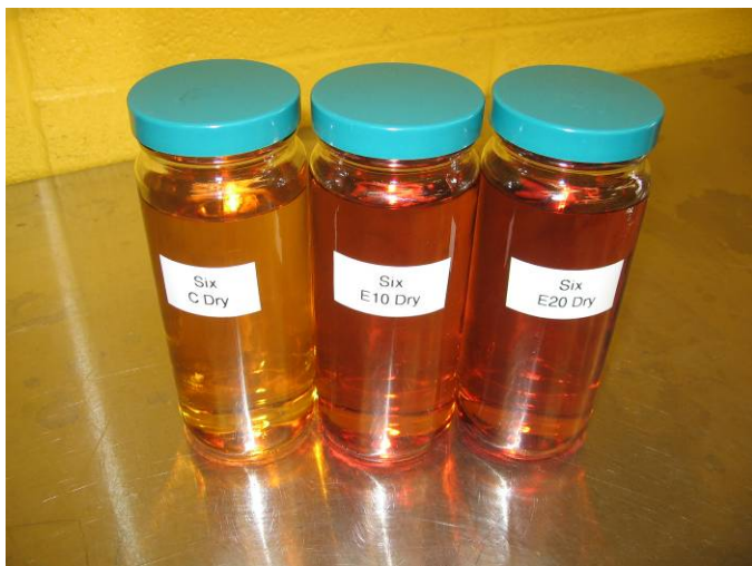
Figure 7. Fluid discoloration from NBR-H after day 1 (Fuel C, left; E10, middle; E20, right)
