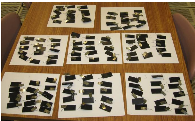
Figure 1. Appearance specimens with ID tags ready for immersion
