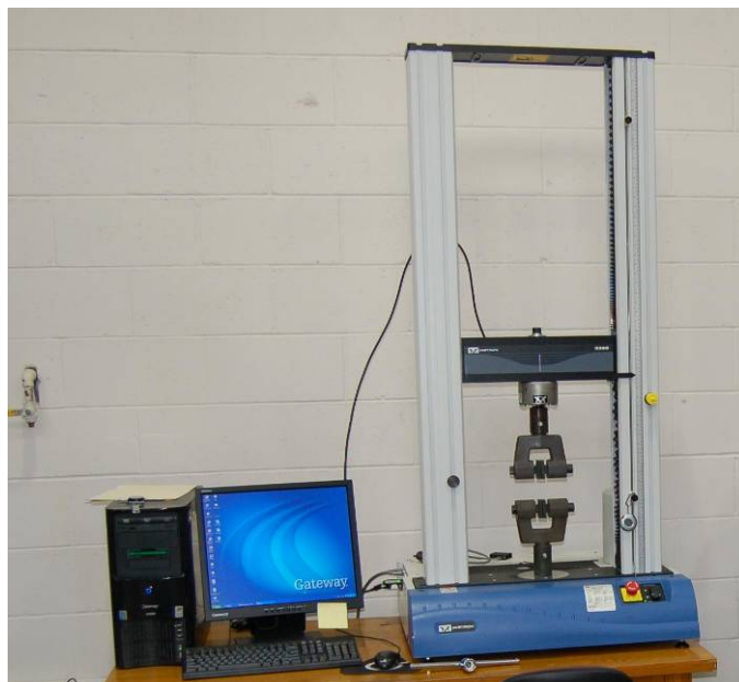
Figure 5. Tensile and Elongation measurement equipment
