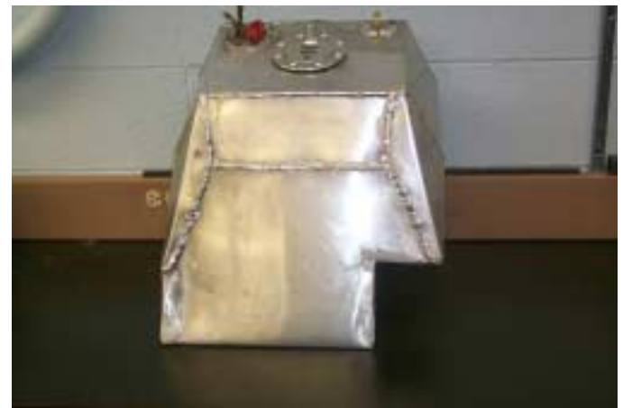
Figure 13 Picture of Mavericks’ Gas Tank
