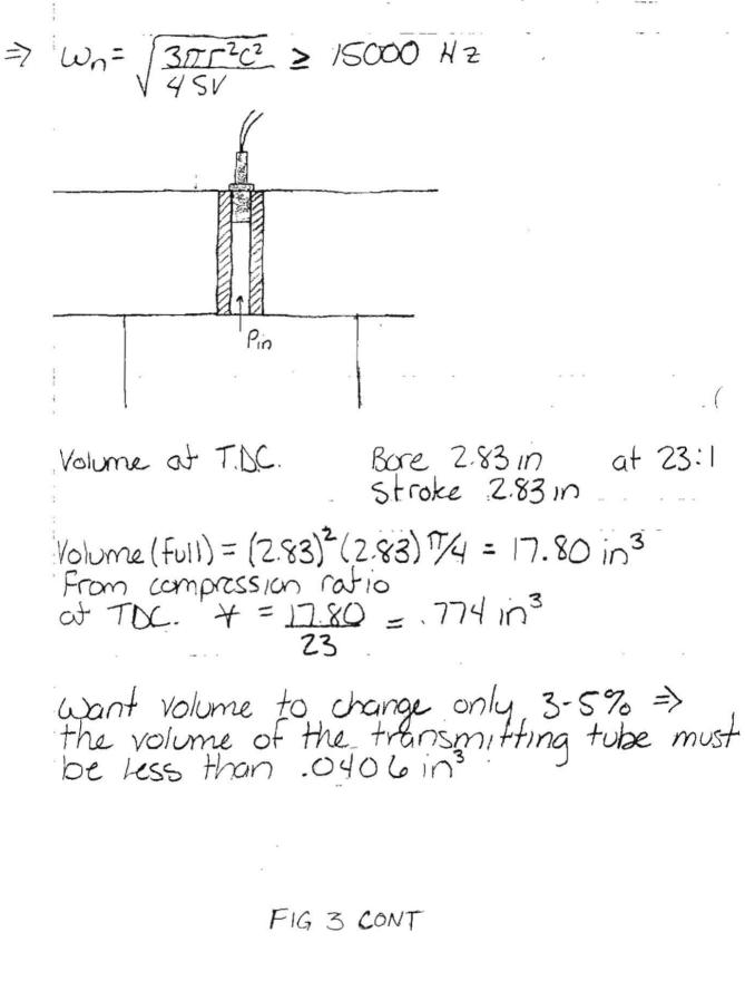
$\omega_n = \sqrt{\frac{3\pi \Gamma^2 C^2}{4SV}}$ . It can be seen that a reduction in the volume tends the wn > 00 Therefore; we will not have an air chamber before the transducer  $\Gamma_{\text{max}} = \sqrt{\frac{V_{\text{max}}}{NS_{\text{max}}}} = \sqrt{\frac{.0400}{N(1.5)}} = .093 \text{ in}$ => \$ max = 3/16" with length at 1.5"
