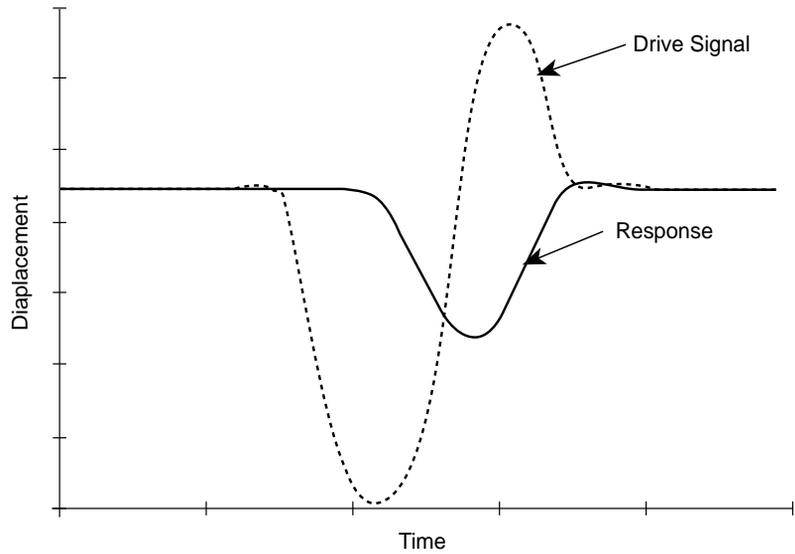
In this UDA command example, you can see the difference between the command, the drive signal, and the feedback.
