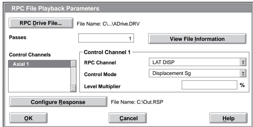
When an RPC III drive file is selected, the Configure Response button is enabled; otherwise, it is disabled. If a response file has not been defined, the response file path is labeled <none>.
