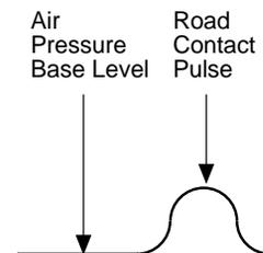
*For example,* suppose you are testing the sidewall of a tire. The base level parameter represents the air pressure in the tire and the height parameter represents the additional force when the sidewall is nearest to the road.
