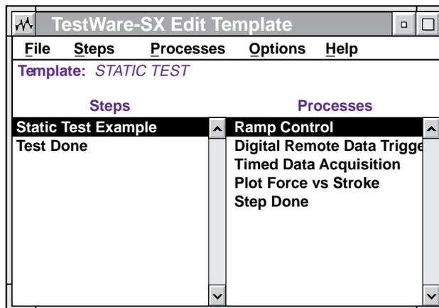
**Note** *If the Ramp Control process is a trigger for the Step Done process when Remote Trigger is enabled, the test step will end prematurely when the first Remote Trigger occurs.*
