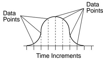
*For example,* suppose you want to acquire data once each 1/100 second. Enter 0.01 second in the Time Increment entry field and select Seconds from the units list icon. Select the input channels you wish to monitor. Data is acquired from all channels each second.
