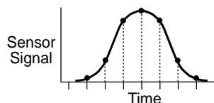
Data is recorded to fill a single buffer once, then stops the process and saves the data to disk.
