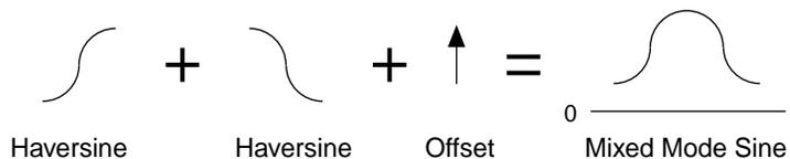
*For example*, suppose you are testing an engine mount. In this case the mean level represents the weight of the engine and the amplitude represents the vibration caused by the engine.
