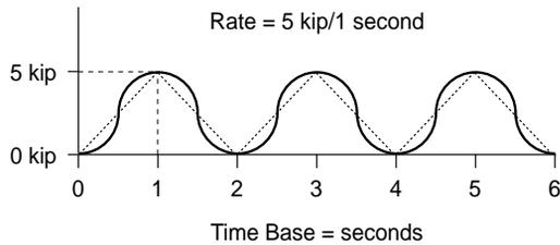
The rate is maintained even though the amplitude has changed.
