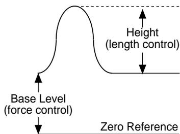
One control parameter can be applied to the height (amplitude) of the pulse while a different control parameter can be applied to the base (mean level) of the pulse
