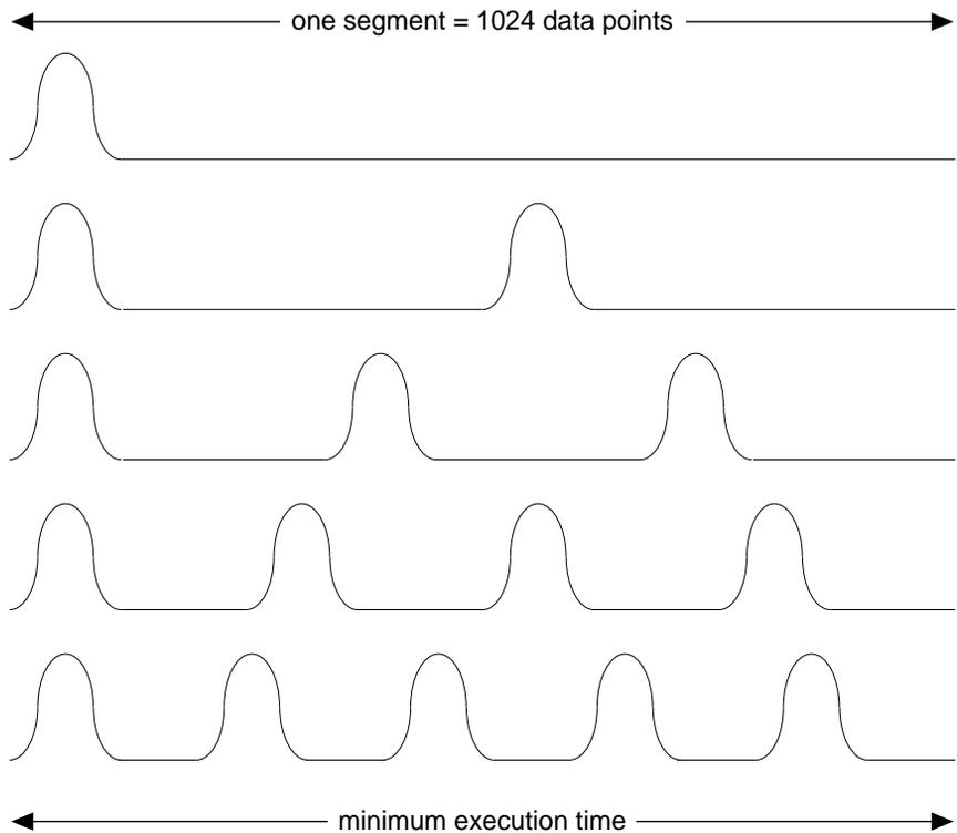
Additional pulses are more likely to be added with higher pulse rates. This can be checked by clicking in another field the new number, if any, is then displayed.
